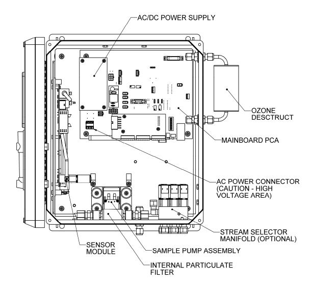
Figure 9-2: Instrument Layout, NEMA Configuration
